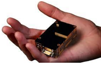
Figure 4-1: Small Form Factor ADS-B/Transponder Mode S with a weight of 190 gr.
