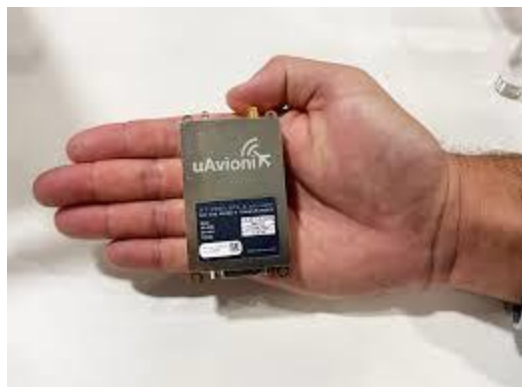
Figure 2-2: IFF Transponder Mode 5 with a weight of 68 gr.
