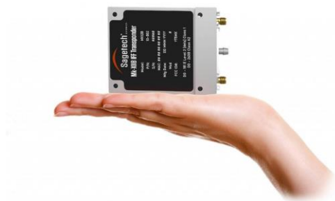
Figure 2-1: IFF Transponder Mode 5 with a weight of 190 gr.
